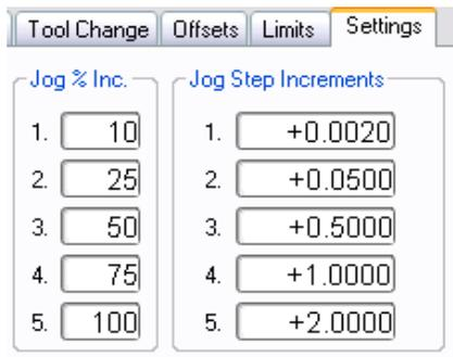
The screenshot shows the 'Settings' tab in the Mach3 software interface. The 'Jog % Inc.' and 'Jog Step Increments' sections are visible. The 'Jog % Inc.' section has five input fields with values 10, 25, 50, 75, and 100. The 'Jog Step Increments' section has five input fields with values +0.0020, +0.0500, +0.5000, +1.0000, and +2.0000.
